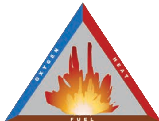
Figure 2.01—The fire triangle. All three components (i.e., oxygen, heat, and fuel) of the triangle must be present for fire to occur.
