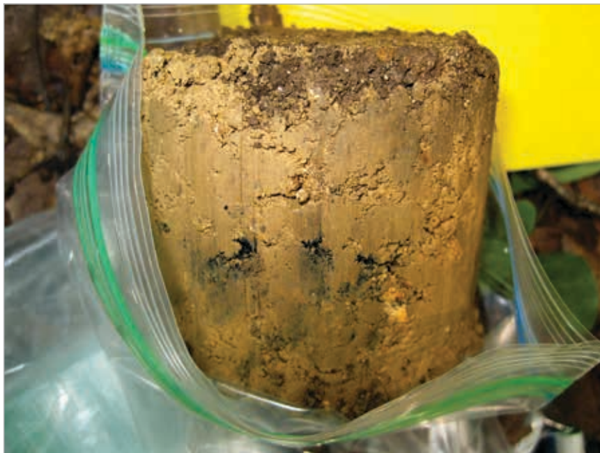
Figure 6.05—Close-up view of a soil core in which charcoal fragments are visible.
