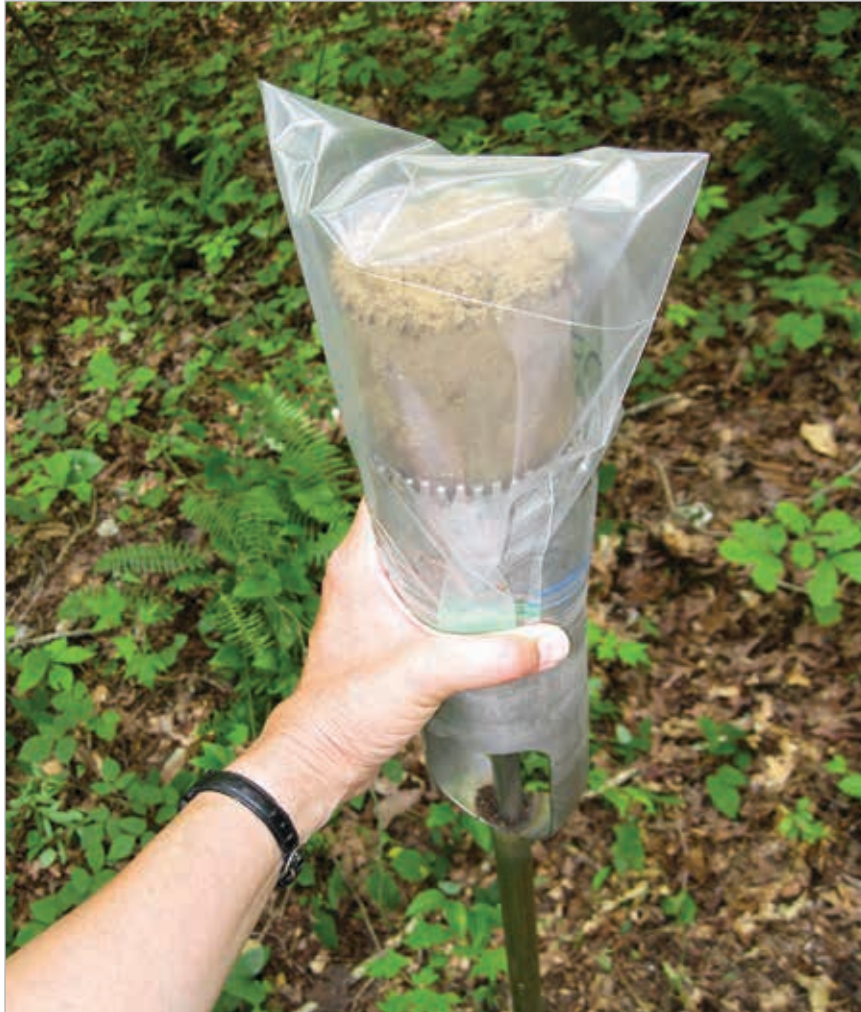
Figure 6.04—Extrusion of a 3.94-inch (10-cm) soil core into a labeled plastic bag.
